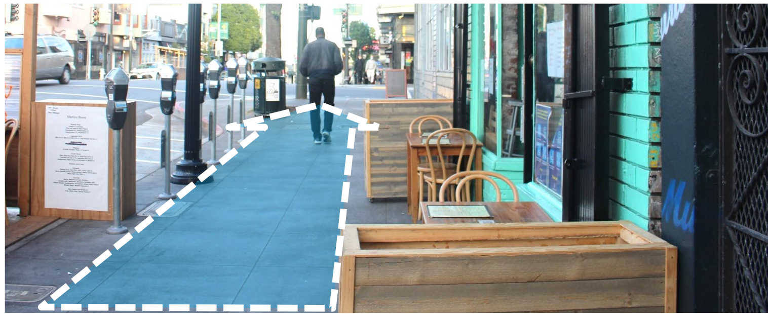
6-foot' Clear Path of Travel, with Diverters
