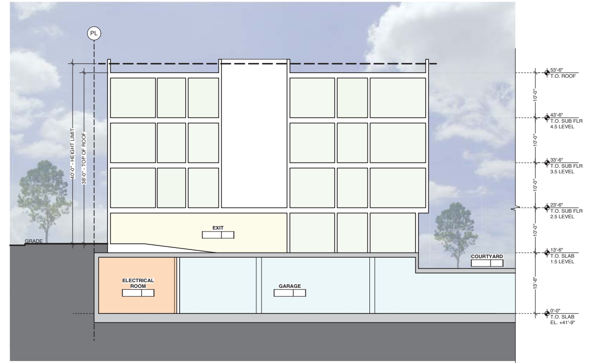
BUILDING SECTION A-A 2 1/8" = 1'-0"
