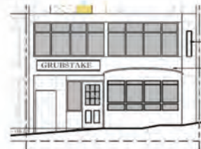
Existing windows including green toplites are being salvaged for reinstallation in the lunch wagon facade
