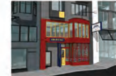
Original: The original design had the arched lunch wagon facade located on the second floor. The facade was at an angle to the property line and did not match the existing footprint.
