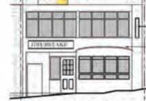
Revised: Existing windows including green toplites are being salvaged for reinstallation in the lunch wagon facade.
