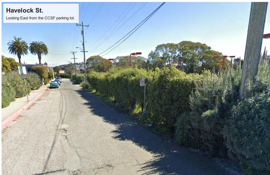
Project will construct approximately 370' of 6.5-foot-wide concrete sidewalk on the south side of Havelock St between the western landing of the Havelock Pedestrian Bridge and the entrance to a parking lot on the City College of San Francisco (CCSF) Campus west of the intersection with Edna St
