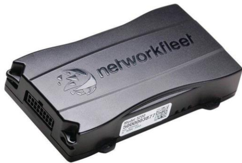
Example of a GPS and cellular tracking device that plugs into a standard vehicle port.
