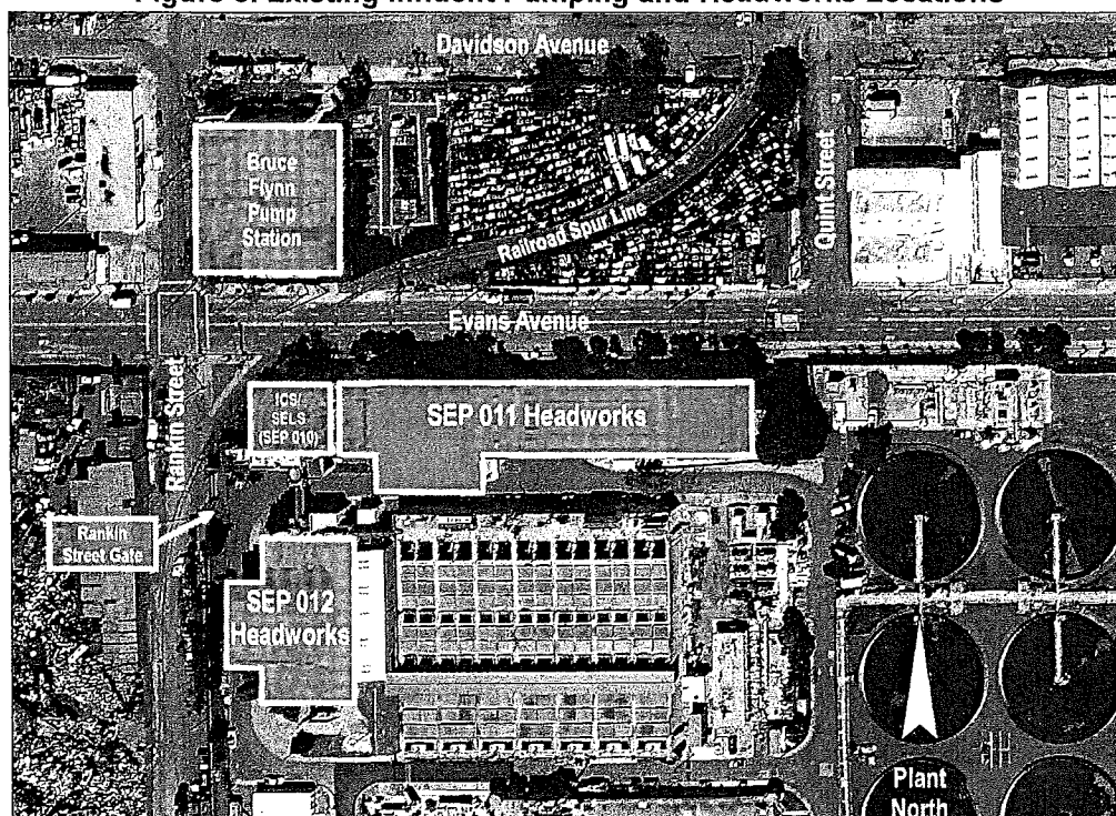
Figure 5: Existing Influent Pumping and Headworks Locations
