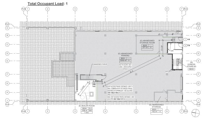
2 BASEMENT FLOOR PLAN - FIRE PROTECTION / EGRESS PLAN SCALE: 1/8" = 1'-0"
