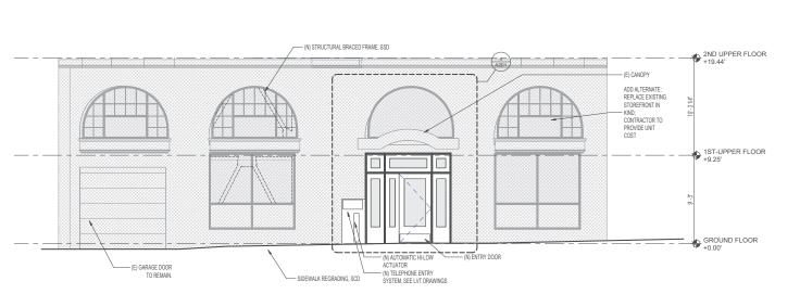
1 ENLARGED ELEVATION - STOREFRONT AND ENTRY SOUTH A2011 SCALE: 1/4" = 1'-0"
