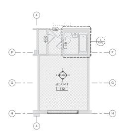
ENLARGED PLAN - TYP EXISITING UNIT 112 - PROPOSED SCALE: 1/4" = 1'-0"
