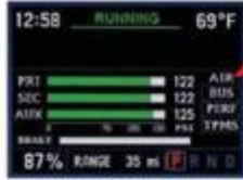
Figure 21-6. Driver Screen Showing Air System Pressures
