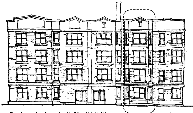
Elevation drawing of a courtyard building. Note that the angled side windows of the bay windows appear narrower because they are not perpendicular to us.
