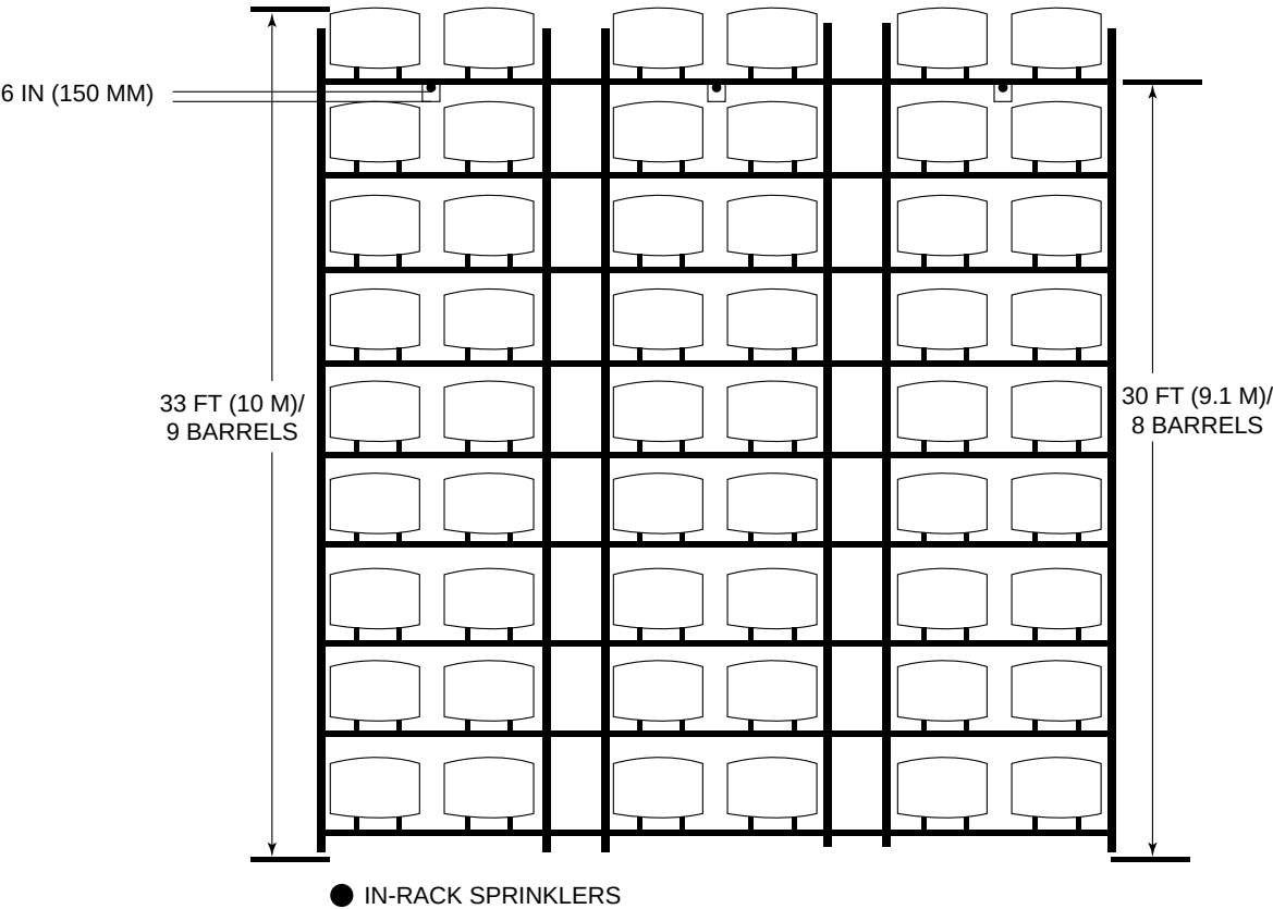
FIGURE 4005.2.3.6(2)—IN-RACK SPRINKLER LAYOUT FOR WOODEN BARRELS ON THEIR SIDES (ELEVATION VIEW)
