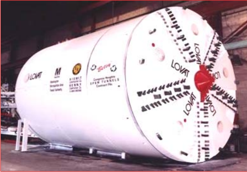
FIGURE 6-1 EARTH PRESSURE BALANCE TUNNEL BORING MACHINE
