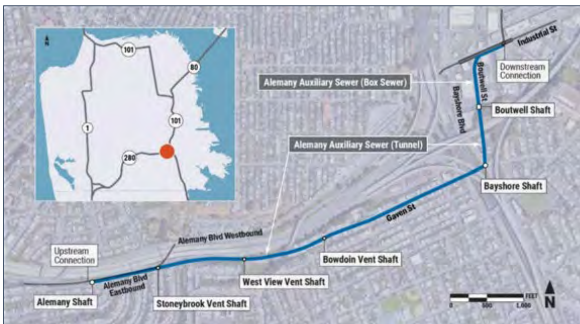
Figure 2. Project Location and Proposed Project Components
