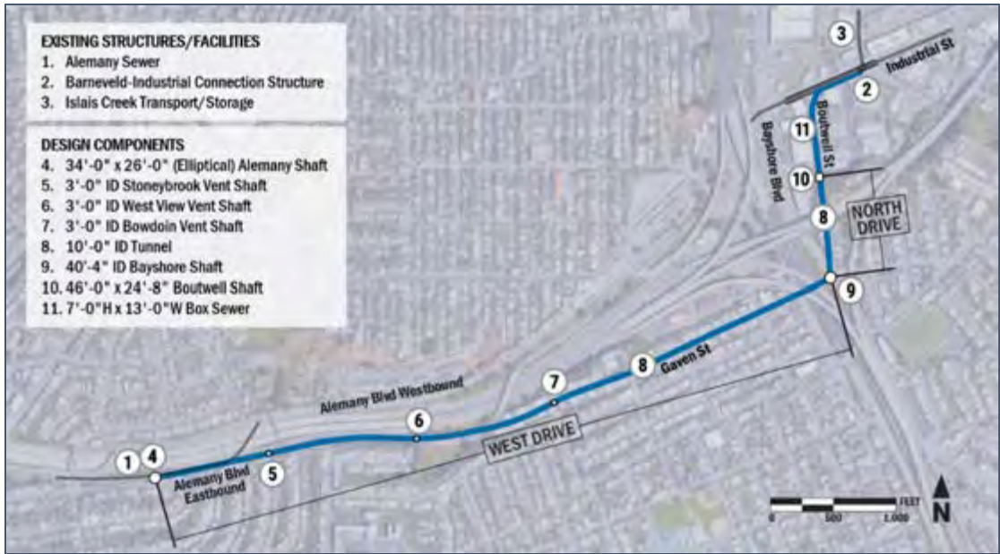
Figure 3. Existing and Proposed Project Components 2
