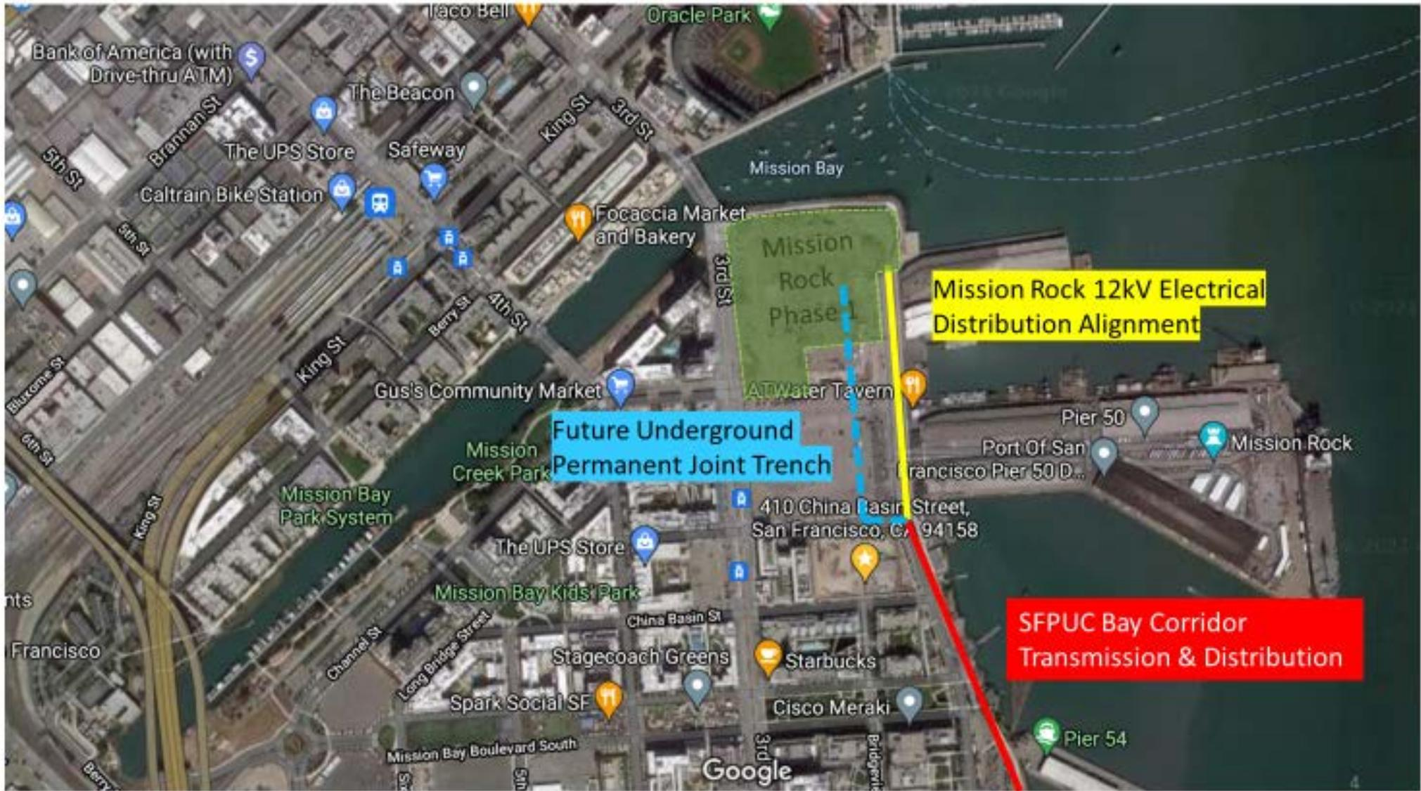
Interim 12kV Electrical Distribution (SIP Ph 1 IB 3/3.1)
