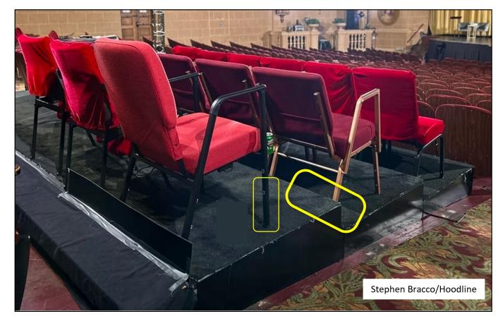
The plans replace 24 rows of 802 permanent seats with 20 rows of ~517 stackable chairs, most sitting on risers with open unprotected front edges, creating trip and fall hazards. People might step off the narrow open edges, especially in the dark. The chairs' protruding front legs create other tripping hazards. Can stackable chairs be secured safely enough for people who struggle with sitting and rising?
