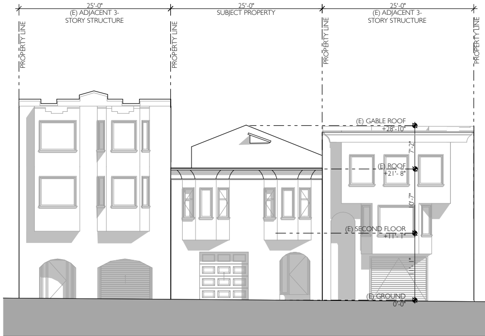
4 (E) EAST (FRONT) ELEVATION SCALE: 1/8" = 1'-0"
