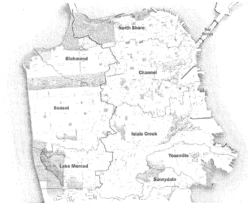
Figure 3. San Francisco is topographically divided into eight individual watersheds.
