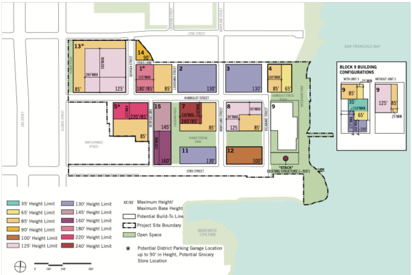
Figure 249.87-4: Building Heights Maximum
