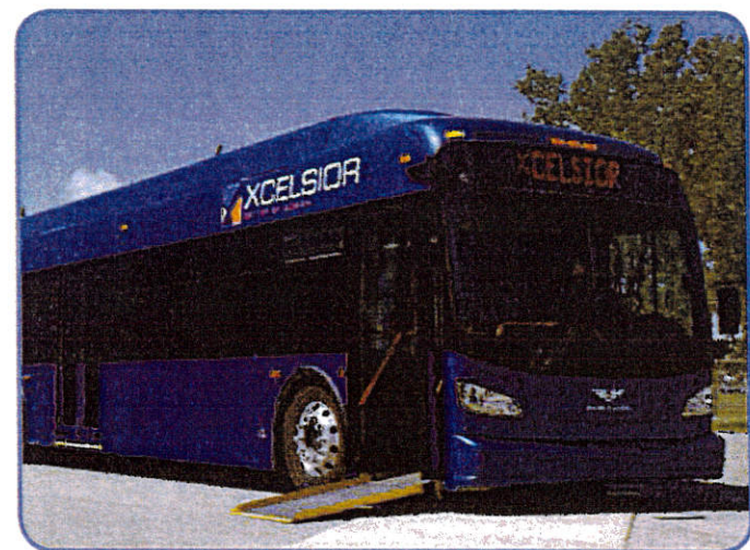
Ramp deployed kneeled (1:7) street level
