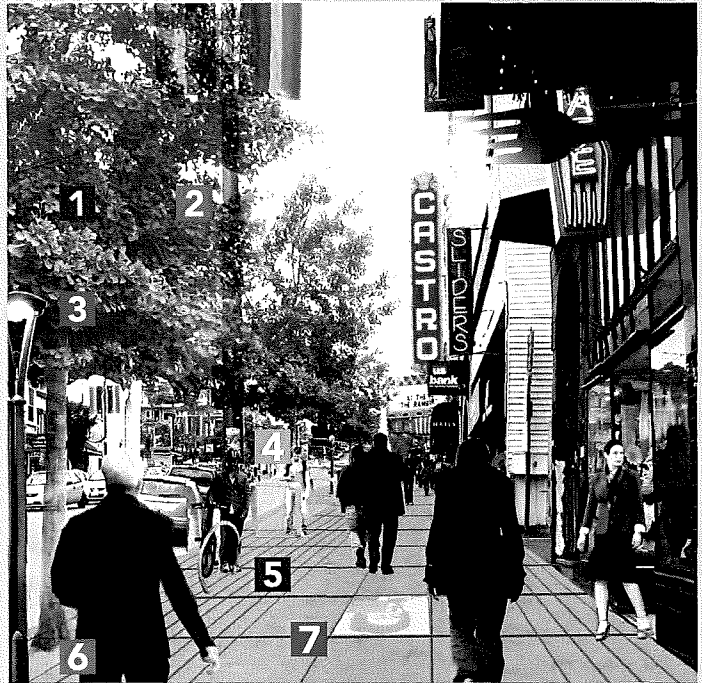
PROPOSED IMPROVEMENTS FOR CASTRO STREET 2014: 1. New Ginkgo Trees planted along curb 2. Relocated Muni and Roadway Light Poles 3. New Pedestrian-Scaled Lighting 4. Leaning Posts 5. New Bike Racks 6. Sidewalks Widened ±10 feet 7. Rainbow Honor Walk Plaques
