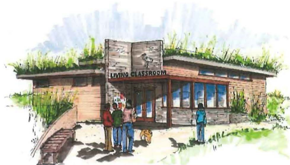
A vegetated roof and other LID features at the Eco-Center at Heron's Head Park help illustrate sustainable design practices to students in San Francisco's Bayview-Hunters Point neighborhood.
