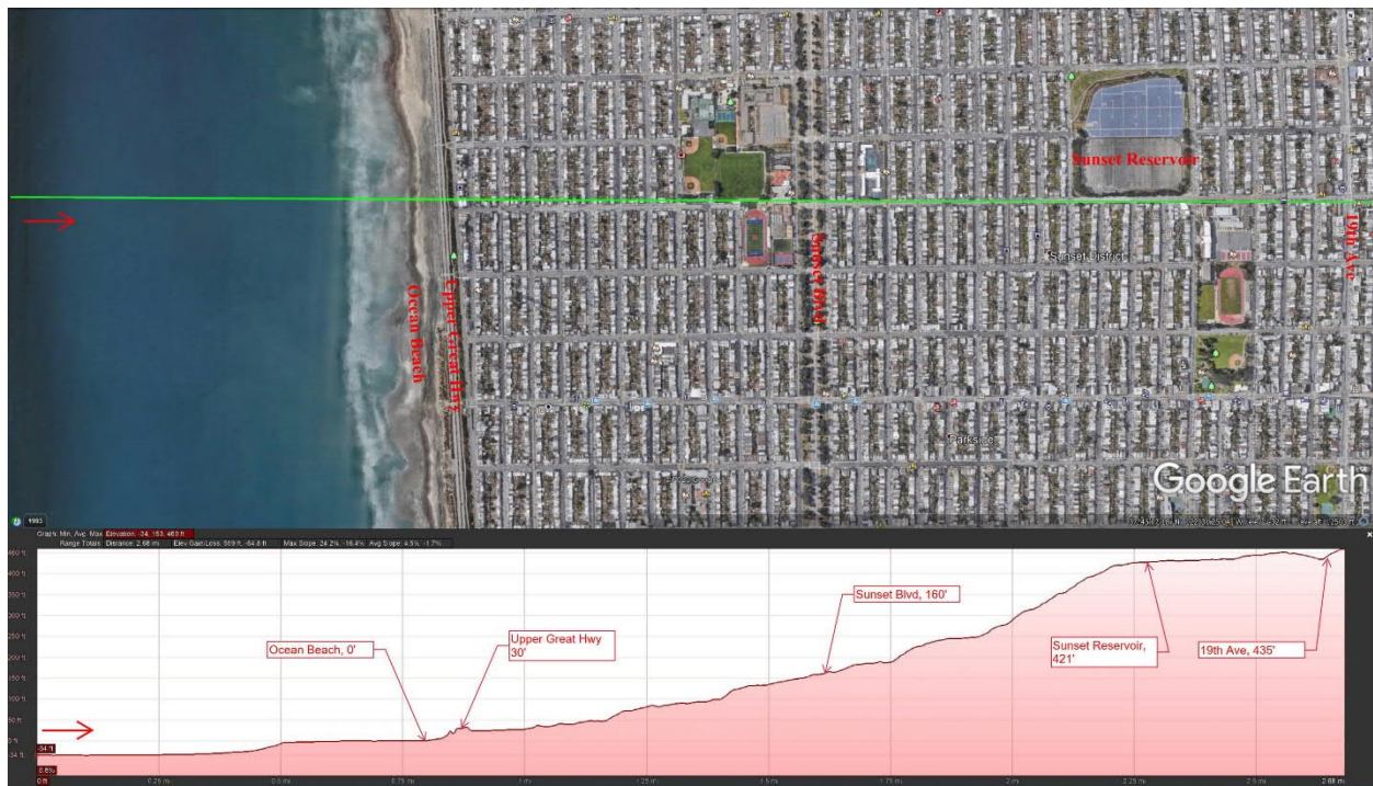
Figure 5-4: Typical Cross Section – Quintara Street/Sunset Reservoir Area
