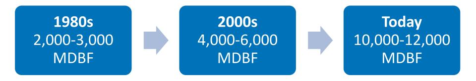
Mean Distance Between Failures (MDBF) is the industry-standard measurement of vehicle reliability. It tracks how long a vehicle travels before an in-service failure
