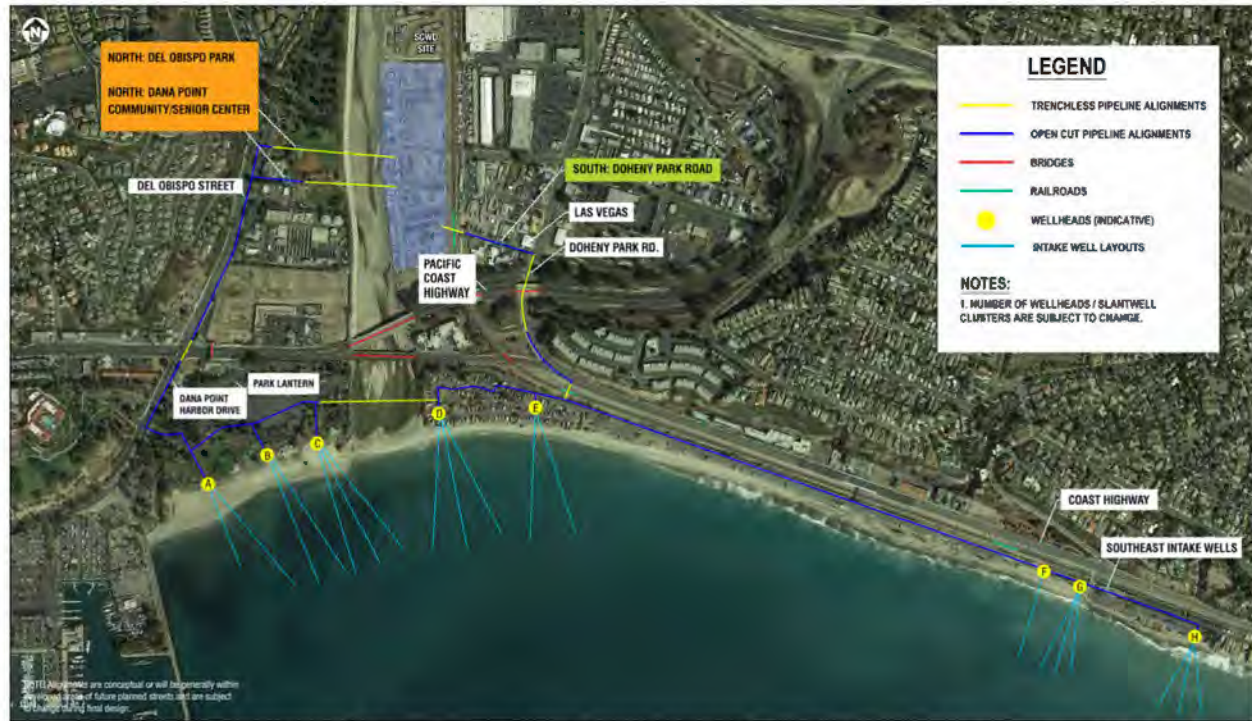
Figure 2-7: Proposed Doheny Desalination Plant Slant Well Intakes
