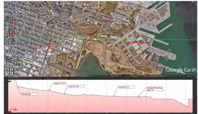
Figure 5-15: Typical Cross Section – Hunters Point Area
