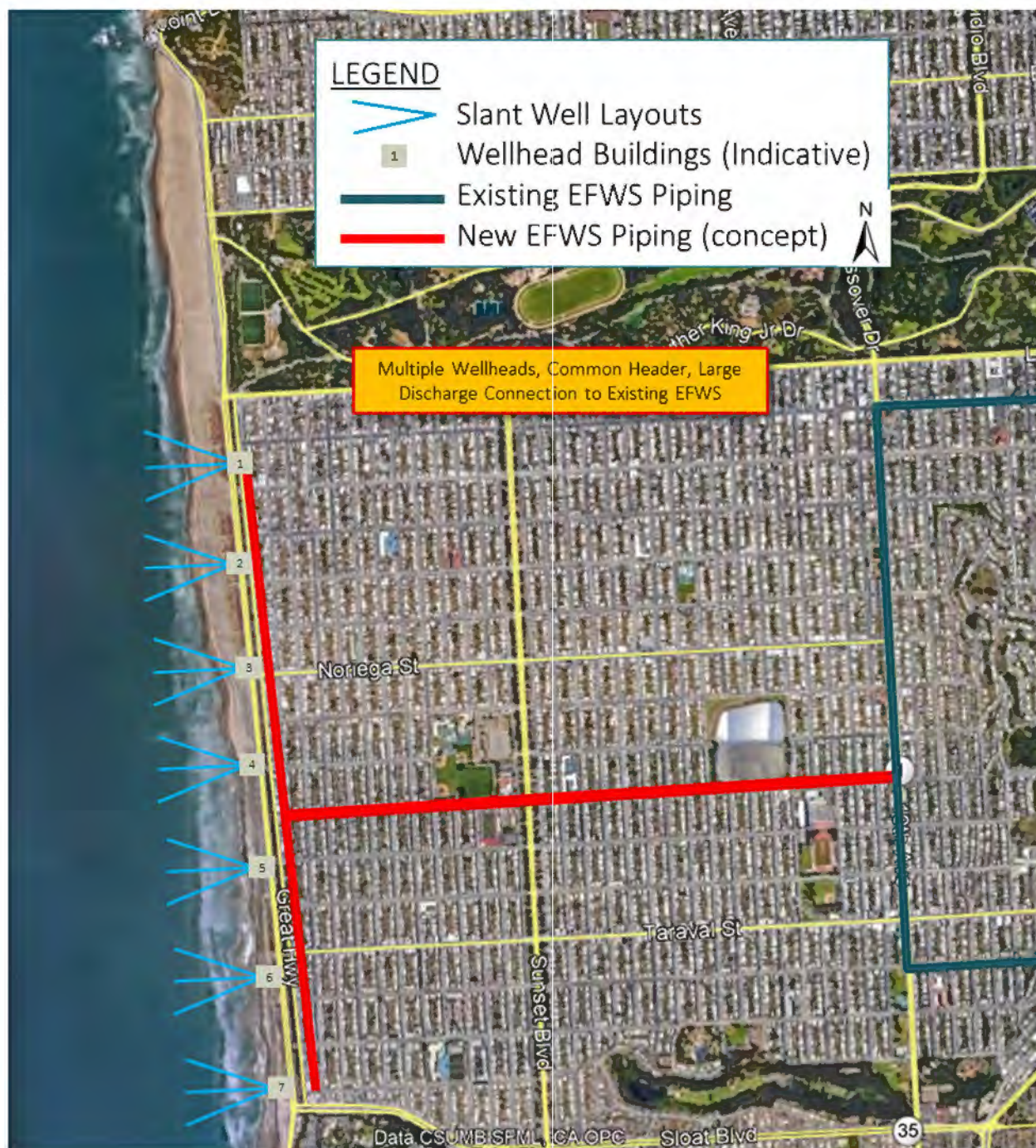
Figure 7-7: Conceptual Layout of Slant Wells at Ocean Beach
