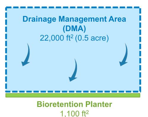
Sizing Ratio = GI Area / DMA = 5%
