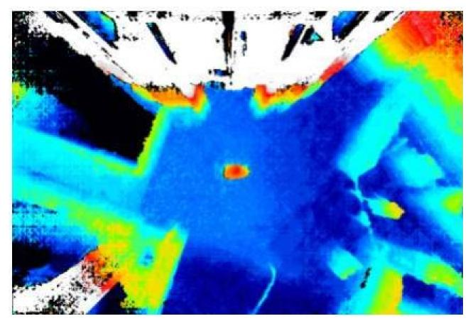
The algorithm analyzes the moving object to see if it fits the known characteristics of a humanoid shape. The red area in the shape of the top of a head. The symmetric orange showing a shoulder shape to the object and then the light green of arms and legs. If it sees these indicators it will consider this to be a trackable object and continue to utilize these height maps to track the object while it is visible to the sensor.
