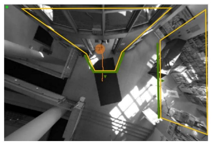
It then tracks the moving object through the scene to see if it crosses a counting line. And then if it meets all of the rules for the count line its count event will be added to the internal storage tally and then the aggregated count data (**not the video images**) is sent to the server in simplified form:
