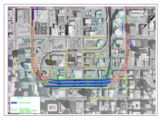
The terminal station would have six tracks and three platforms and would include approximately 2,000 feet of additional tracks (called tail tracks) in a cut-and-cover section leading from the east end of the new Terminal. These tracks would curve 90 degrees south along 498-foot to 521-foot
