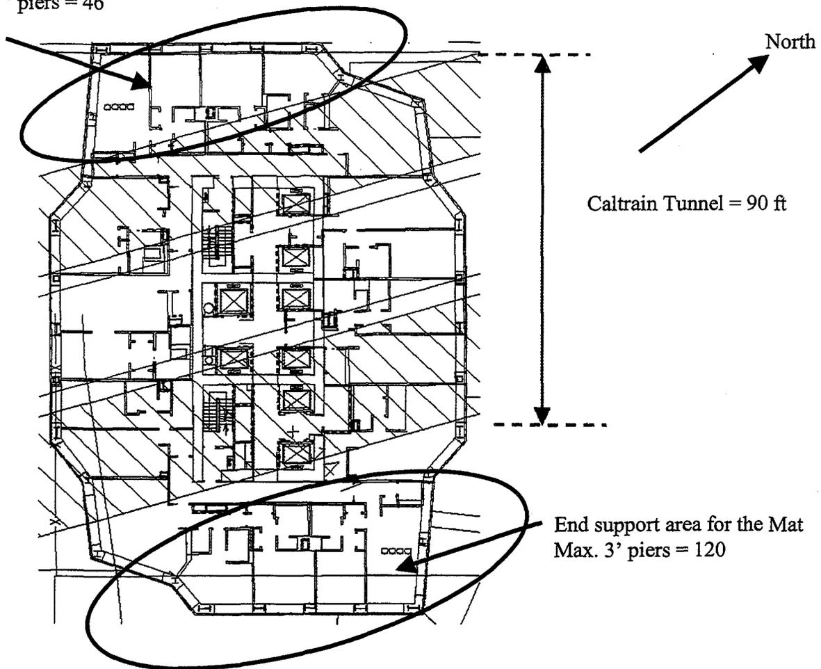
Figure 1: Building Foot Print Overlaid with Caltrain Tunnel
