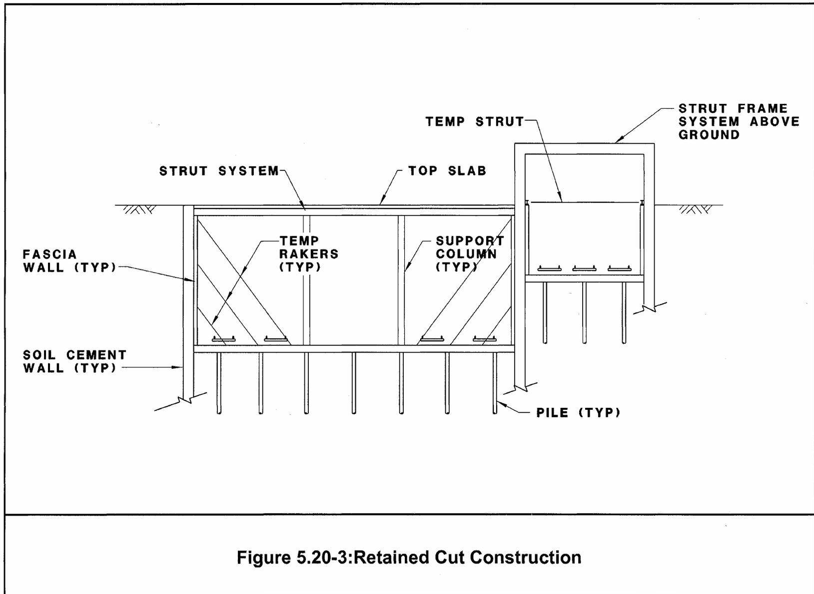
Figure 5.20-3: Retained Cut Construction
