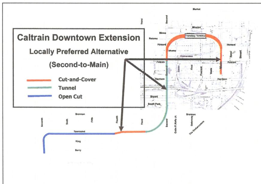
Street and continue underneath Main Street to south of Folsom Street. The tail tracks could also be extended as a separate, independent project at some time in the future, to a San Francisco-to-Oakland cross-bay alignment for commuter rail and/or high-speed trains. *This Second-to-Main*
