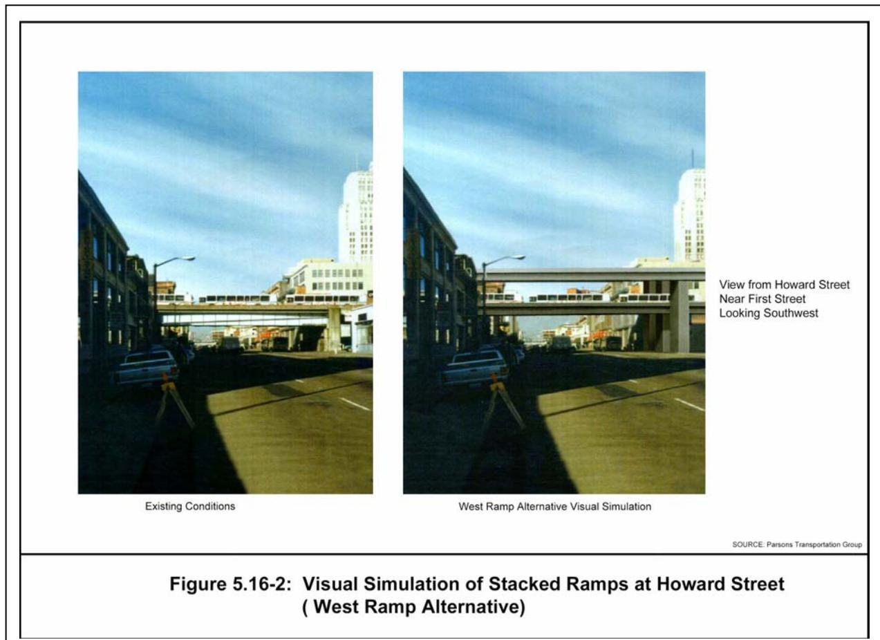
The proposed ramps would occupy considerably less area than the existing ramps, and would be split, breaking up the mass of the ramps and allowing views between the two new ramp sections. Although the new decks would be approximately 30 feet tall, they would be less visually intrusive due to their uniform appearance and minimal supporting structures.
