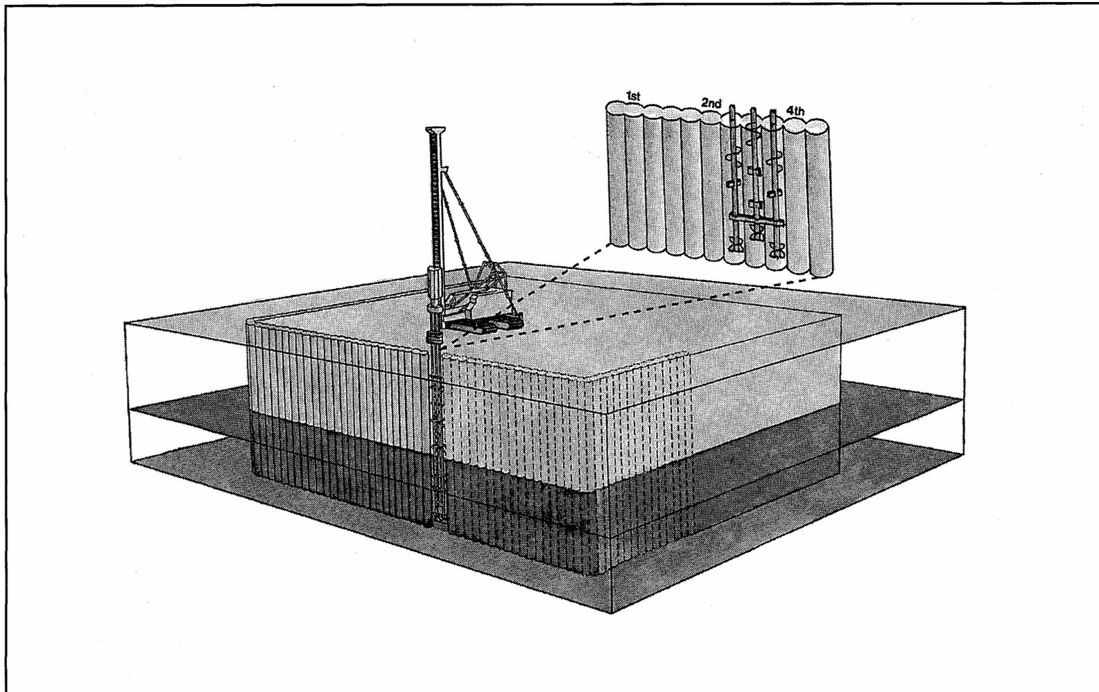
Figure 5.20-2: Column Construction for Soil Cement Walls
