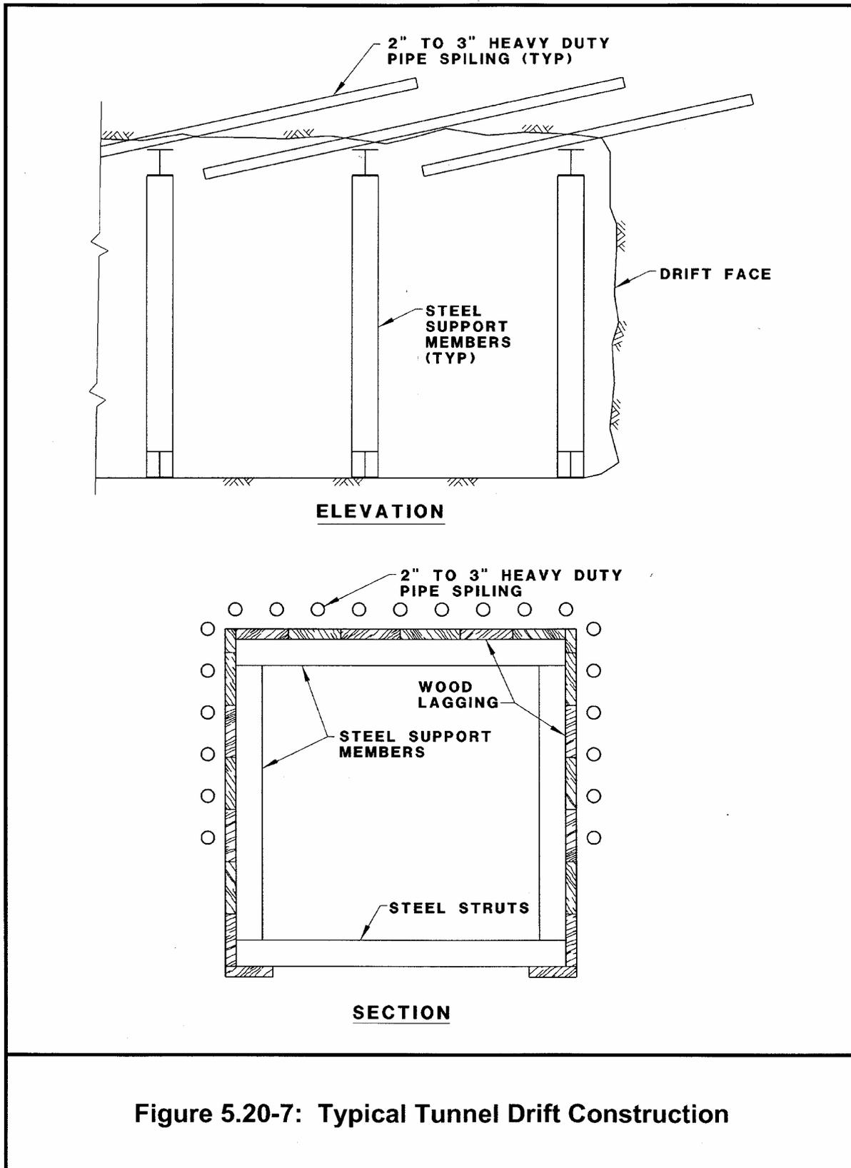
Figure 5.20-7: Typical Tunnel Drift Construction
