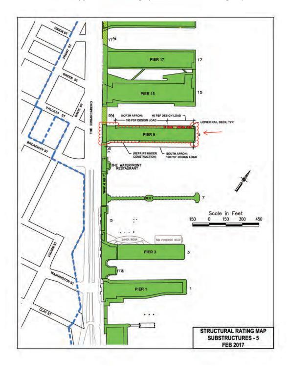
Photo 16. Substructure rating map updated for Pier 9 only.
