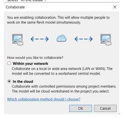
4. When prompted navigate to the appropriate discipline folder and save the cloud workshared model – confirm that the file name is in line with conventions set out in the BIM Execution Plan. <ENTER RDC FILE STRUCTURE IMAGE>
