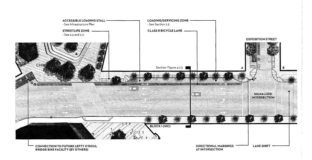
A northound buffered bicycle lane would provide commuters an alternative to traveling through China Basin Park to connect to a planned two-way cycle track across Lefty O'Doul Bridge.
