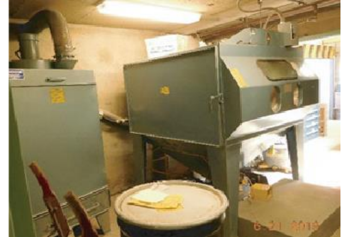
Old B-Blasters in most shops in confined space with inadequate ventilation. No containment of debris.
