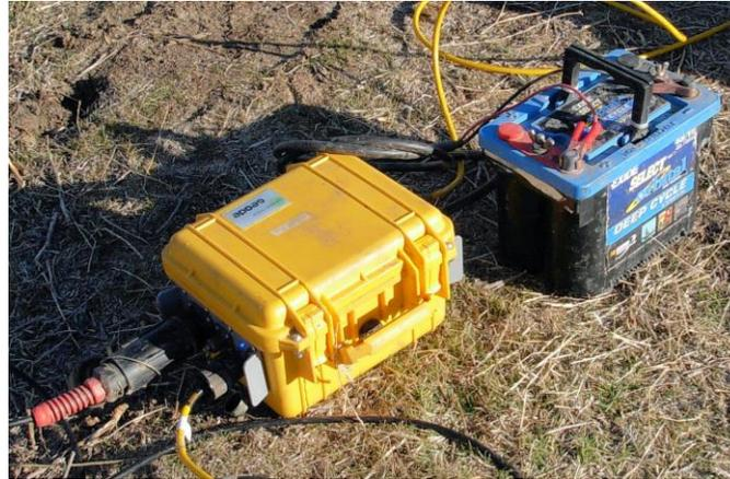
**Figure 1:** Geometrics Geode 24-channel engineering distributed array seismograph.
