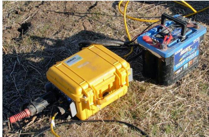
**Figure 1:** Geometrics Geode 24-channel engineering distributed array seismograph.
