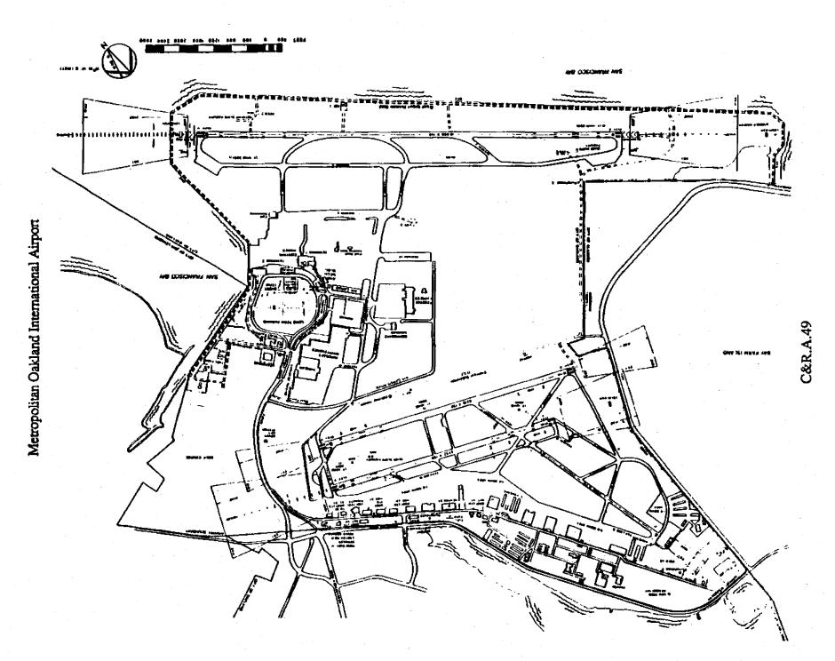
6,212 feet long and 150 feet wide; 9L-27R, which is 5,452 feet long and 150 feet wide; and 15-33, a short crosswind runway which is 3,366 feet long and 75 feet wide. The air carrier runway, 11-29 at South Field is approximately 6,400 feet from the closest general aviation runway, runway 9-27. There is one designated helicopter takeoff/landing area.
