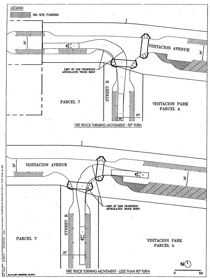
FIGUR 27 17 JENLARGEMENT OF TYPICAL INTERSECTION FIRE TRUCK TURNING
