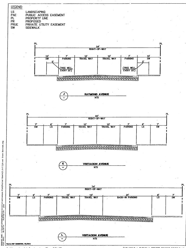
FIGURE 7.6: TYPICAL STREET CROSS SECTIONS
