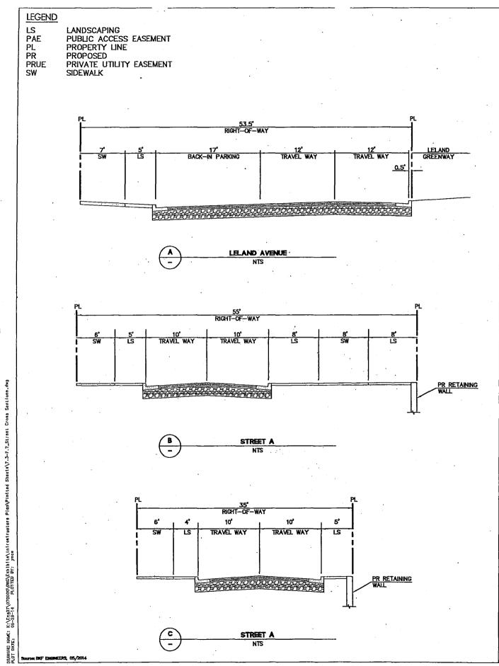
FIGURE 7.3: TYPICAL STREET CROSS SECTIONS
