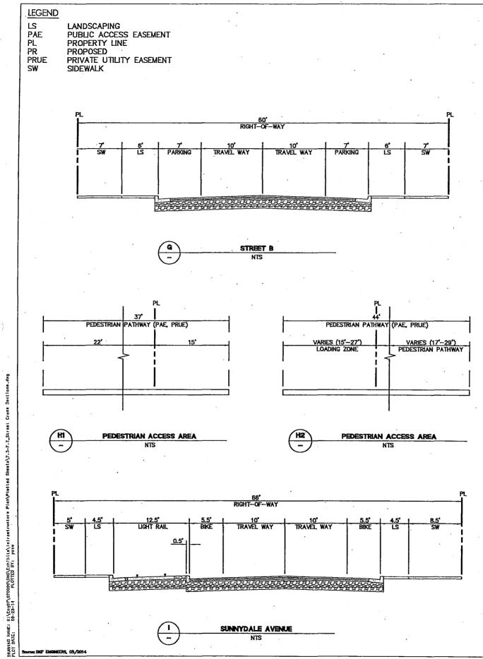
FIGURE 7.5: TYPICAL STREET CROSS SECTIONS
