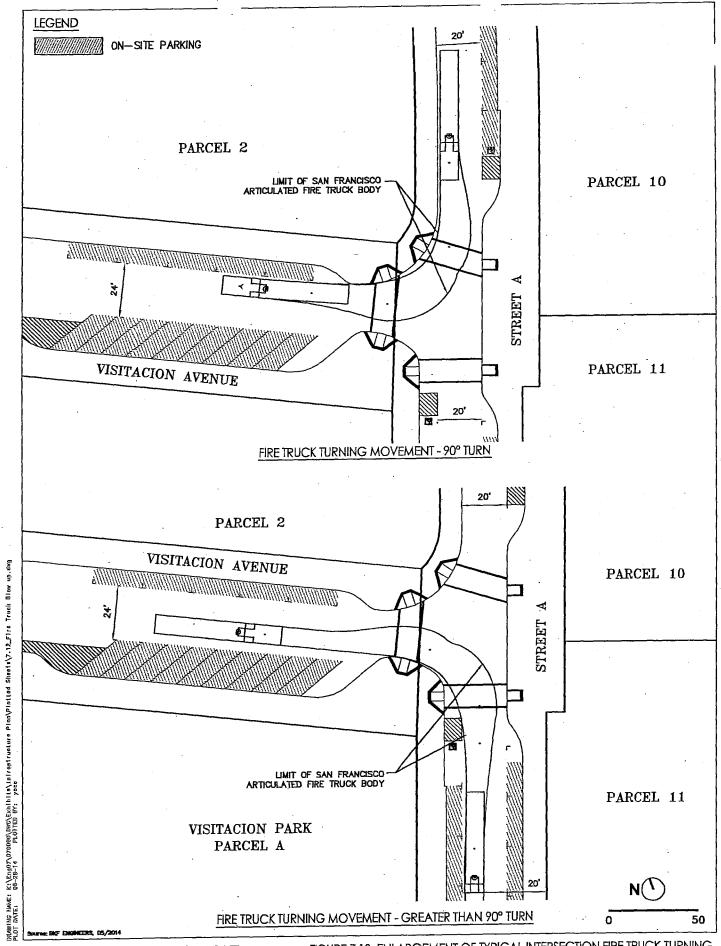
FIGURE 7.12: ENLARGEMENT OF TYPICAL INTERSECTION FIRE TRUCK TURNING 2176
