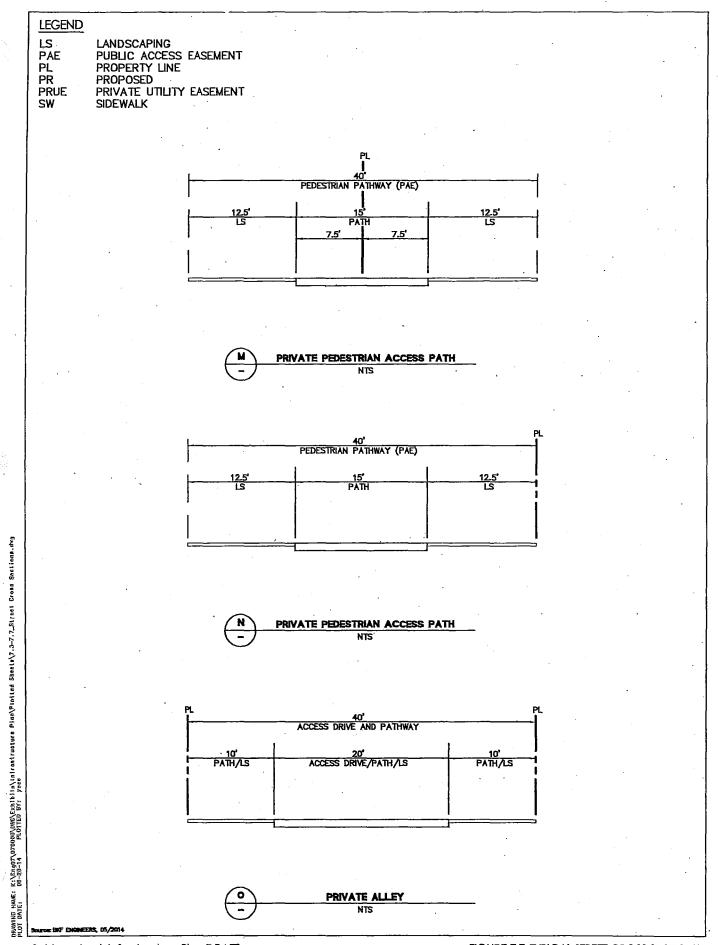
FIGURE 7.7: TYPICAL STREET CROSS SECTIONS
