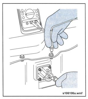
Fig. 56: ESS Voltage Check Between HV Terminals & Ground
