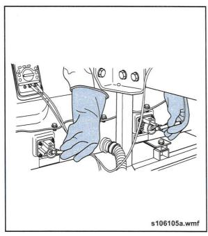
Fig. 55: ESS Voltage Check Between HV
