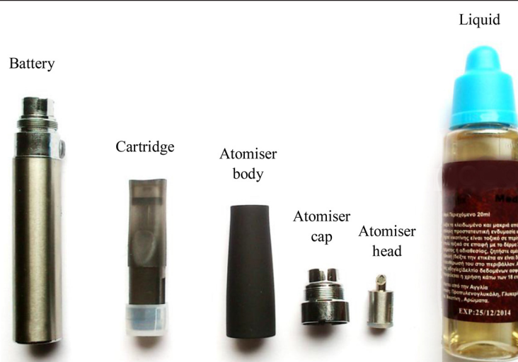
Figure 1 Electronic cigarette device and liquid used in the study.
