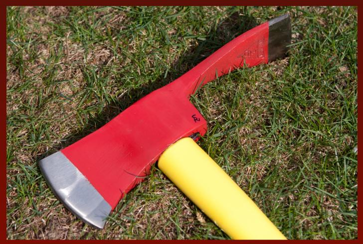
Pulaski; The tool combines an <u>axe</u> and an <u>adze</u> in one head with a rigid handle of wood, plastic, or fiberglass. The pulaski is a versatile tool for constructing <u>firebreaks</u>, as it can be used to both dig soil and chop wood.
