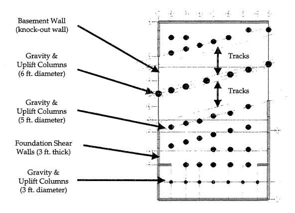
Figure 3: Foundation Plan Layout
