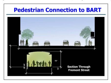
Figure 2.2-24: Pedestrian Connection to BART (Conceptual Cross Section)
