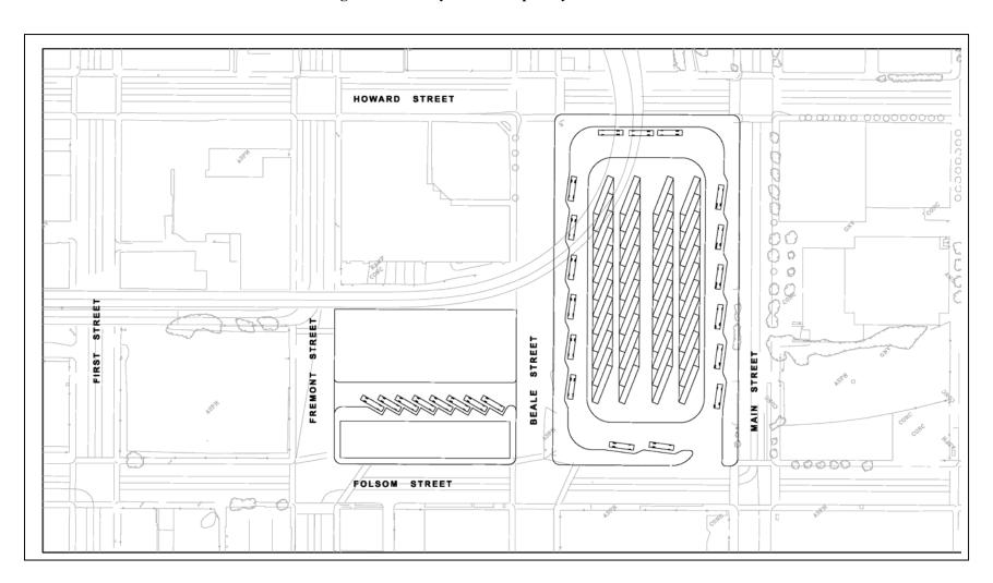
Figure 2.2 8: Layout of Temporary Bus Terminal
