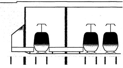
Section through terminal showing side platform
