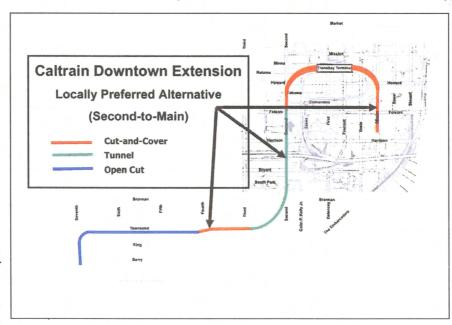
Street and continue underneath Main Street to south of Folsom Street. The tail tacks could also be extended as a separate, independent project at some time in the future, to a San Francisco-to-Oakland cross-bay alignment for commuter rail and/or high-speed trains. *This Second-to-Main*
