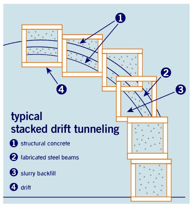
Figure 5.20-6: Stacked Drift Tunnel Construction
