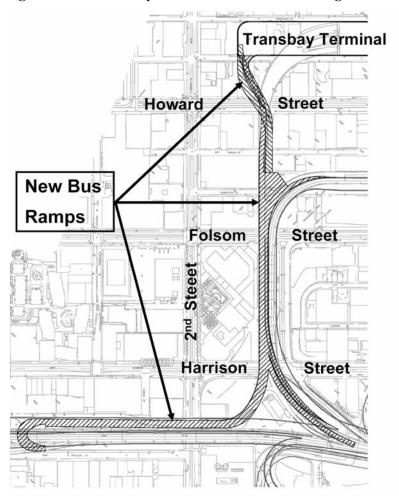
Figure 2.2-4: Transbay Terminal Off-Site Bus Storage Link Ramp
