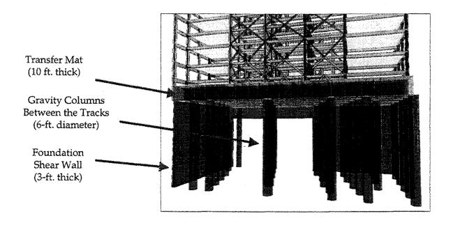
Figure 2: 3-D model of below-grade structure
