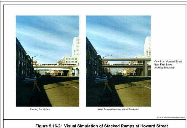
Figure 5.16-2: Visual Simulation of Stacked Ramps at Howard Street (West Ramp Alternative)
