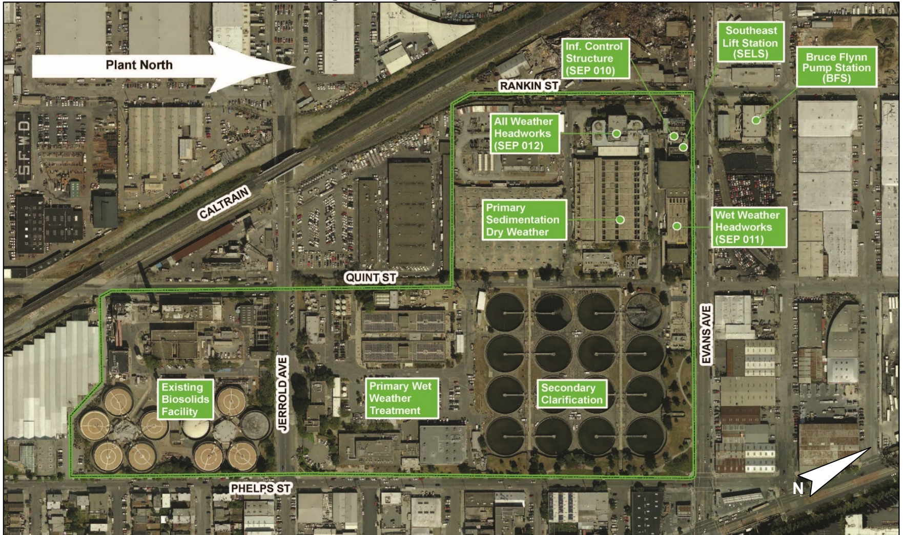
Figure 2: Existing Southeast Plant Site
