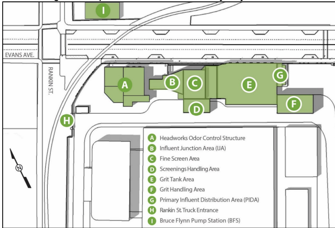
Figure 7: Proposed New Headworks Facility Project Site Plan
