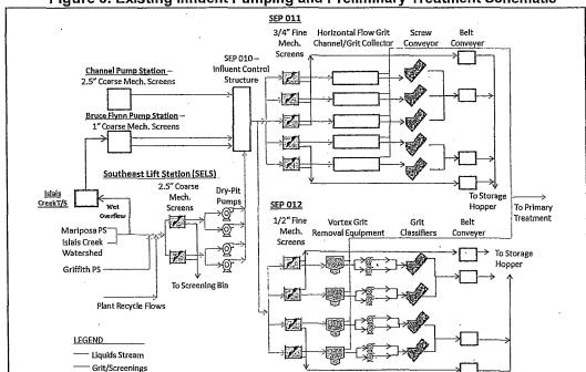
Figure 6: Existing Influent Pumping and Preliminary Treatment Schematic
