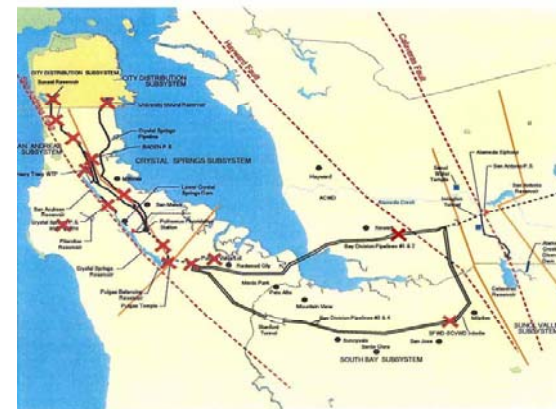
Figure 10. SFPUC Facilities Assumed to Fail in the Event of an Earthquake on the San Andreas Fault (Red Xs Indicate At-Risk Facilities)
