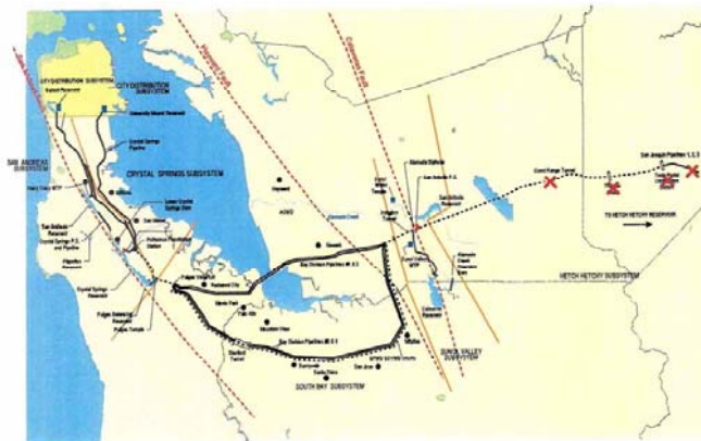
Figure 13. SFPUC Facilities Assumed to Fail in the Event of an Earthquake on the Great Valley Fault (Red Xs Indicate At-Risk Facilities)
