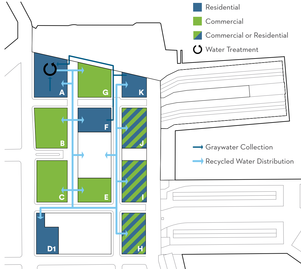
FIGURE 2.4: Graywater Collection and Reclaimed Water Distribution Infrastructure
