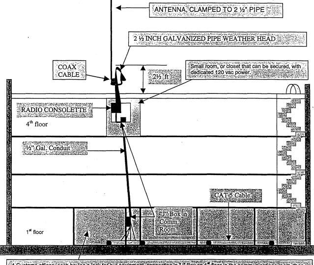
4 Customs offices, each having a jack for our equipment, connecting in "J". Box on 1<sup>®</sup> floor in the communications room, then to top floor radio comm. closet:
