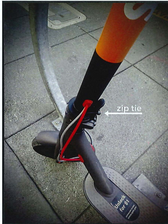
Competitor's attempt to ensure that the scooter handle is not foldable by using a zip tie.
