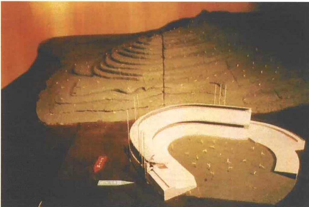
Figure 1 Original Candlestick Park wind tunnel test model
