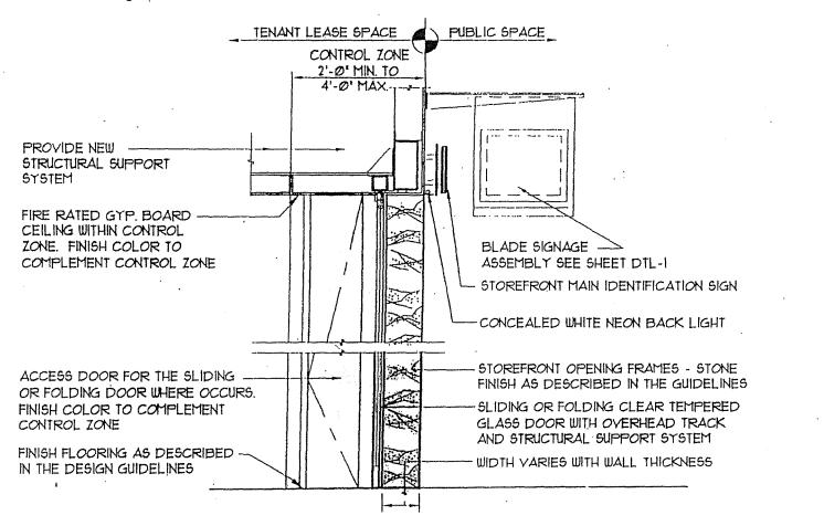
**WALL SECTION - CONDITION #1** Scale:  $1/2^{"} = 1' - 0"$
