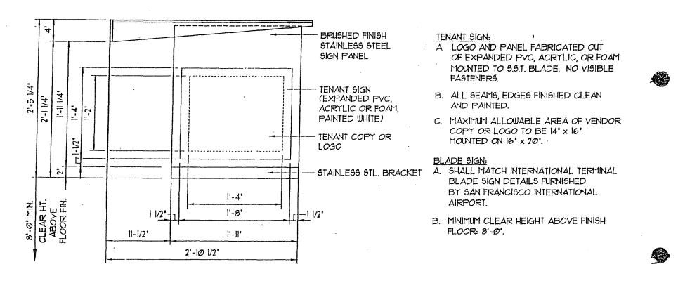
**BLADE SIGN ELEVATION** Scale:  $1^{"} = 1^{-0"}$
