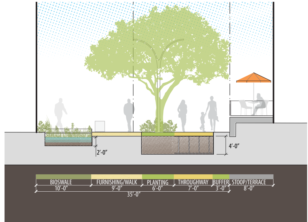
FIGURE 2.29: COVE LANEWAY SECTION-TYPICAL
