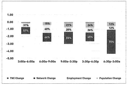
**Figure 23** shows the decrease in average speeds between 2010 and 2016, as well as the share of this delay caused by different factors. The decline in average evening speeds has been most precipitous, dropping over 4 miles per hour, with almost 75% of this change attributable to TNCs. Speed decreases during the other time periods were about 3 miles per hour, with about 45%-55% of this decrease caused by TNCs.
