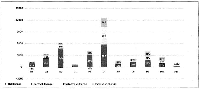
**Figure 27** illustrates the total increase in delay between 2010 and 2016, as well as the share of this delay caused by TNCs, network changes, population changes and employment changes. The greatest increases in delay occurred in Districts 3 and 6, with approximately 73% of the increase in delay in District 3 due to TNCs, and about 45% of the increase in delay in District 6 due to TNCs. We estimate that approximately 36% of total delay in District 3 and District 6 combined is due to TNCs.
