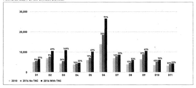
**Figure 26** compares the delay from 2010 to the 2016 No TNC scenario in which TNCs don't exist, and to the 2016 with TNC scenario. This figure shows that TNCs increased delay in all districts relative to 2016 No TNC scenario. The greatest total increases in delay occurred in District 3 and District 6. The greatest relative increase in delay occurred in District 3, while the greatest total amount of delay occurred in District 6.
