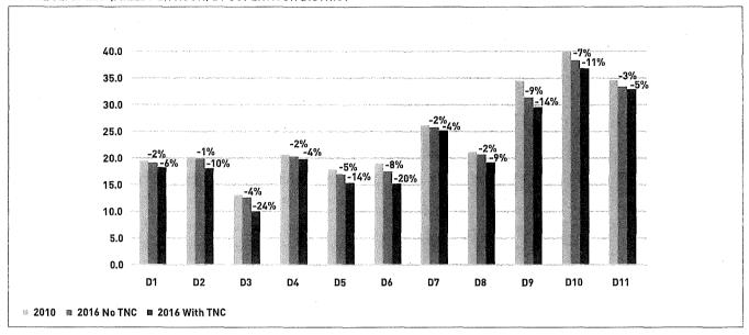
**Figure 32** compares speeds from 2010 to the 2016 No TNC scenario in which TNCs don't exist, and to the 2016 with TNC scenario. The percentage change shown is relative to the 2010 Base scenario. This figure shows that average speeds have declined in all districts, with the greatest relative declines between the 2016 No TNC and 2016 With TNC scenarios occurring in Districts 3, 6, 5 and 9. Overall speeds were lowest in District 3 and highest in District 10.
