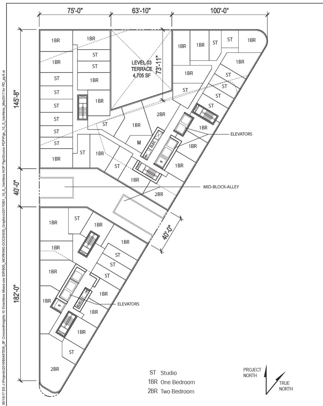
Figure 10: Proposed Project – Representative Floor Plans for Levels 3–12
