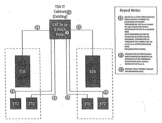
Figure 2 illustrates all of the equipment that must be connected to the IDF IT cabinet for a CBIS where the EDS machines are already networked together. When the EDS machines are networked together (i.e., MUX, NEDS, etc.), the connection only needs to be made to the EDS Network Server(s).
